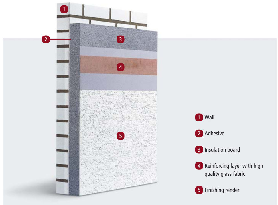
A thermal insulation composite system consists of insulating material and various types of coating.
