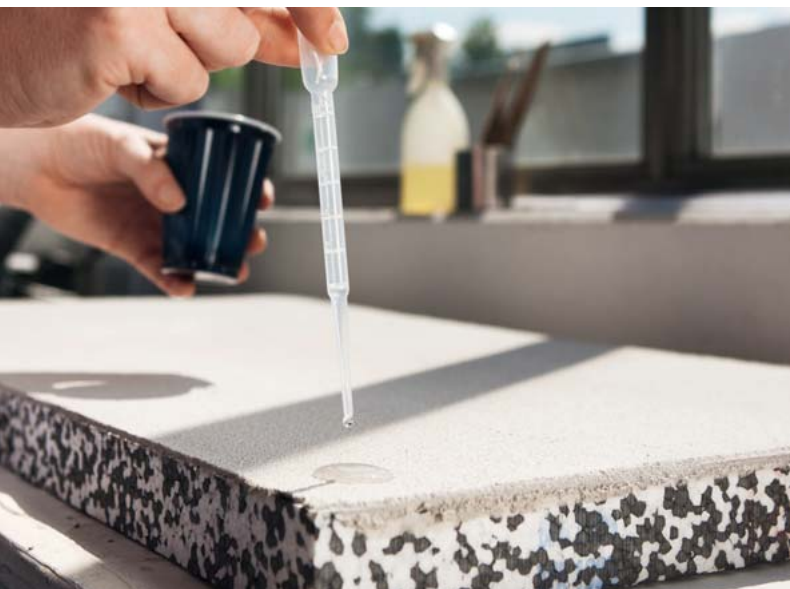
Water-repellent: The coating of the Capatect Dalmatiner facade insulation fulfilled high demands during testing.
